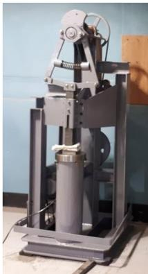
(a) Remodeled machine(spring hammer)[16]
