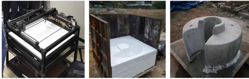
[Fig. 3] Form Liner Manufactured by LOM[13]
