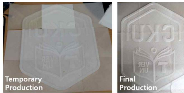
[Fig. 8] Disposable Form Liner Printed by 3D Printer
